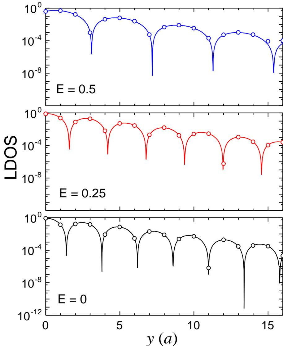
Layer-dependent DOS using parameters extracted from the complex band structure
