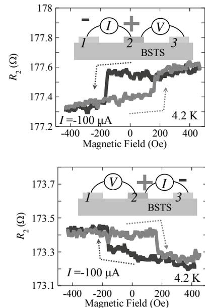
Fig. 1 Results of magnetoresistance measurement in Py/BSTS devices measured at 4.2 K.
