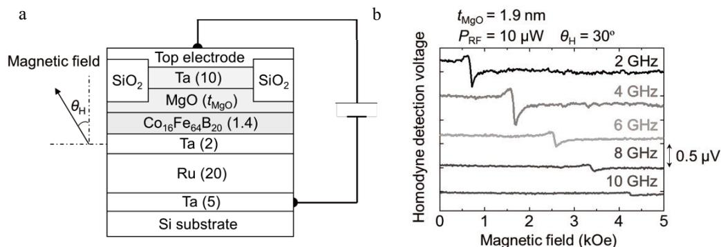
Figure 1 (a) Device structure. (b) Typical FMR spectra of CoFeB detected by TAMR.
