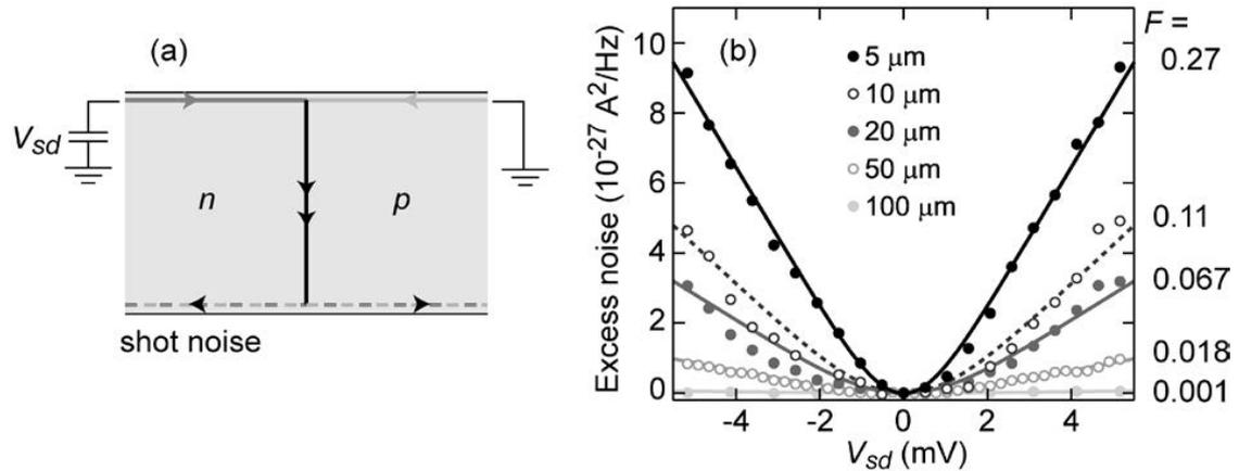
Figure 1: (a) Mode mixing and partitioning in a graphene  $p$ - $n$  junction in quantum Hall effect regime. (b) Shot noise as a function of  $V_{sd}$  for five samples with different length of the  $p$ - $n$  junction. The filling factors in the  $p$  and  $n$  regions are  $\nu = -2$  and  $2$ , respectively. The magnetic field is  $10 \text{ T}$  and the temperature is  $4 \text{ K}$ .
