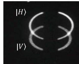
Fig. 1 Optical image of the SPDC
