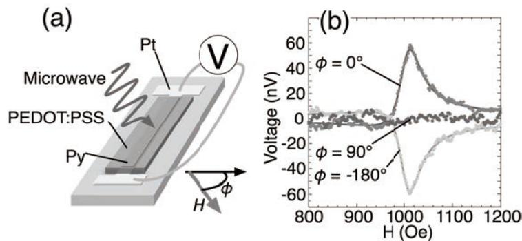
Figure 1: (a) Schematic of the sample structure used for the spin pumping experiment. (b) Magnetic field dependence of the voltage signal in Py/PEDOT:PSS/Pt trilayer for  $\phi = 0^\circ$ ,  $90^\circ$ , and  $180^\circ$ .
