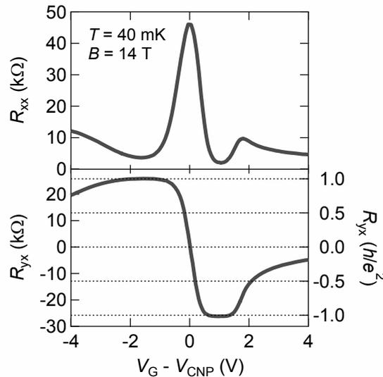
Fig.1: QHE with  $\nu = \pm 1$  observed in (Bi<sub>1-x</sub>Sb<sub>x</sub>)<sub>2</sub>Te<sub>3</sub> film ( $x = 0.84$ )
