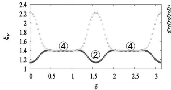
Figure 1: The lowest four ES  $\xi_\nu$  for each phase  $\delta$  of the modulation of the chemical potential. The amplitude is  $0.5t$  and the wave length is  $4a$ , where  $t$  is the hopping integral and  $a$  is the lattice constant. The number enclosed by a circle represents the degeneracy of the lowest levels of the ES.
