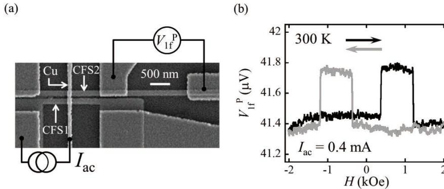
Fig 1: (a) SEM image of a fabricated LSV for the spin-Peltier measurements. (b) Field-dependent nonlocal voltage detected by the Cu thermocouple on the CFS2 wire at 300K under electrical spin injection at  $I_{ac} = 0.4$  mA.
