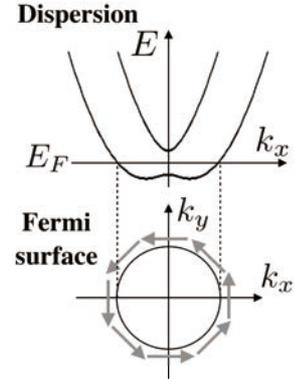
Fig.1: The energy dispersion and the spin structure on the Fermi surface in the helical metal.
