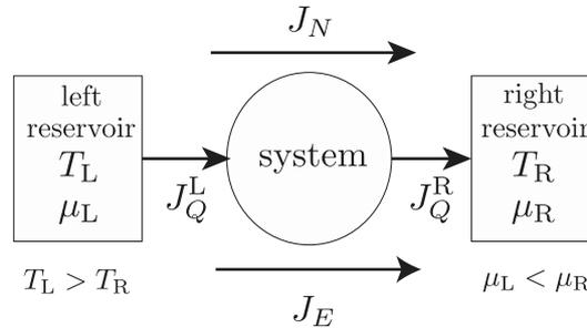
**Figure 1. A mesoscopic thermoelectric engine.**
