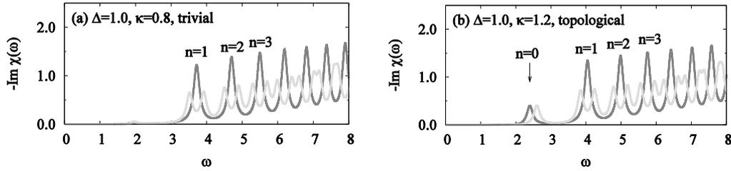
Figure 1: Imaginary part of the dynamic spin susceptibility of a 2D Dirac system with spin-orbit interactions [red (green): without (with) Zeeman effect]. An anomalous peak appears only in the topological phase.
