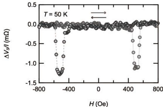
Fig. 1 A nonlocal spin valve signal measured at 50 K.
