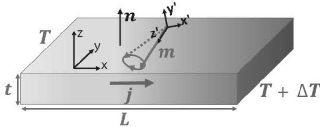
Figure 1: Single-domain magnetization dynamics induced by microwave field pumps magnon and spin currents by virtue of Dzyaloshinskii-Moriya interactions. This can develop a temperature gradient along the sample. Alternatively, a temperature gradient can result in magnon current and torque on uniform magnetization according to the Onsager reciprocity principle.
