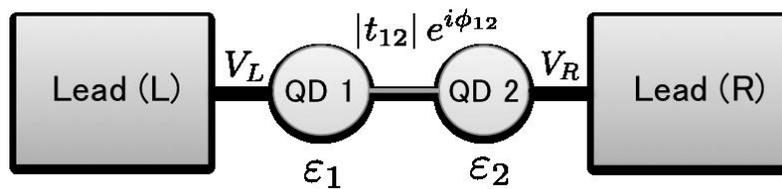
Figure 1: quantum dot coupled to two reservoirs with time-dependent modulating parameters.
