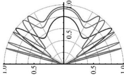
Figure 1: (Color online) angular dependence of quantum transport of an excitation with energy  $\varepsilon/\Delta = 2, 3, 4$  corresponding to red, brown and blue curves, respectively. We set  $\Delta=10$  meV and  $v_D = 10^5$  m/s. The length of junction is  $L=1\mu\text{m}$ .
