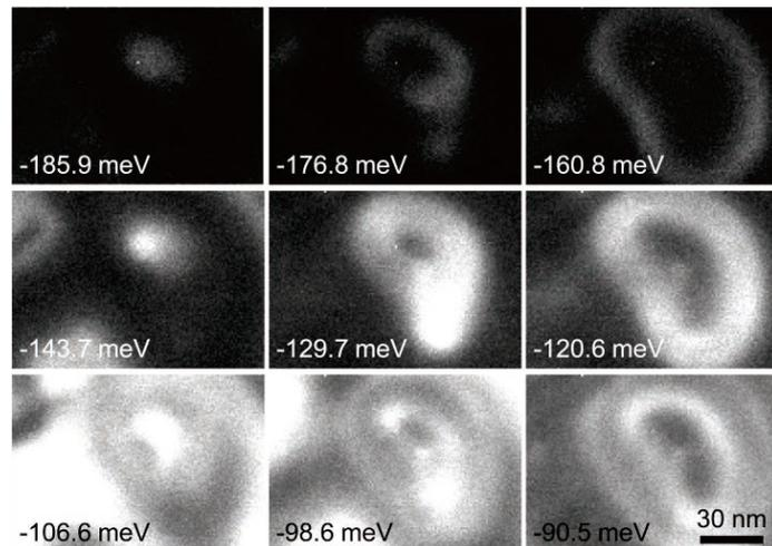
Figure 1: LDOS distributions in the topological surface state of  $\text{Bi}_2\text{Se}_3$  at 11 T, showing the Landau orbits drifting around the potential minimum. Top, middle and bottom rows correspond to  $n = 0, 1$  and  $2$  states, respectively [1].
