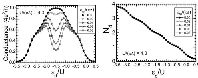
Figure 1: NRG results of (left) conductance and (right) average of  $N_d$  for Coulomb repulsion  $U/(\pi\Delta) = 4.0$  and zero field  $b = 0$ , are plotted vs  $\varepsilon_d$ , for several different orbital splittings  $\varepsilon_{\text{sp}}/(\pi\Delta) = 0.00, 0.02, \dots, 0.08$ . Typical energy scale is  $T_K/(\pi\Delta) \simeq 0.13$ .
