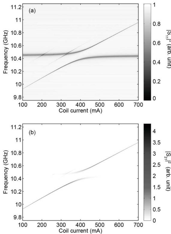
**Figure 1:** Spectroscopy of the coupled system consisting of the microwave cavity and the Kittel mode coupled system. (a) Spectrum probed by microwave reflection, and (b) those probed via Faraday effect.
