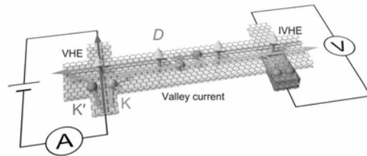
Figure 1: Schematic image of the pure valley current mediated nonlocal transport
