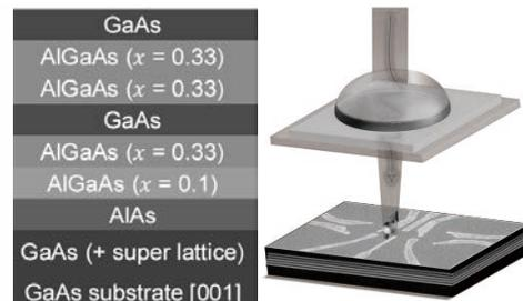
Fig. 2 Layer structure of the wafer (left) and fine pattern fabrication (right)
