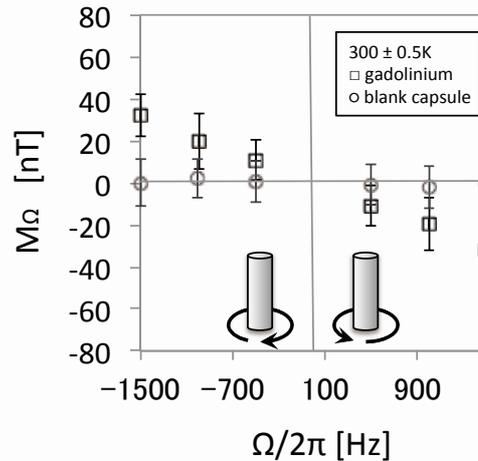
Figure 2: Rotational frequency dependence of the magnetization observed at  $300 \pm 0.5$  K for the Gd sample and the blank capsule. Each data point is averaged over three measurements with the error bar in the standard deviation  $1\sigma$  including the rotational frequency fractionation.
