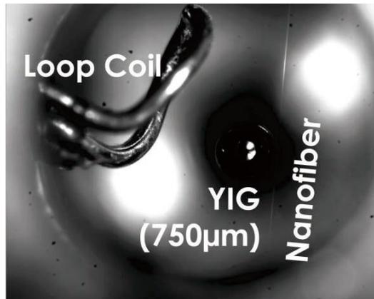
Fig. 1 Spherical optical resonator made of a ferrimagnetic YIG. YIG sphere is optically coupled via the nanofiber and magnon is excited by microwave.
