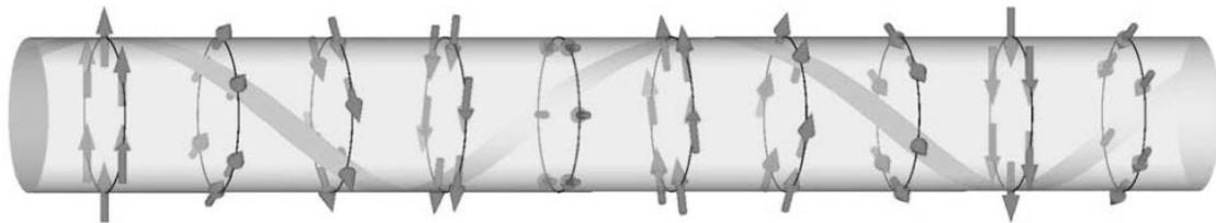
Figure 1: One dimensional conductor (yellow) with helically oriented spins (red).
