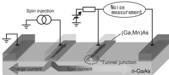
Figure 1: Schematic diagram of the measurement system.
