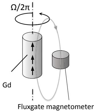
Figure 1: The experimental setup for observation of the Barnett effect.
