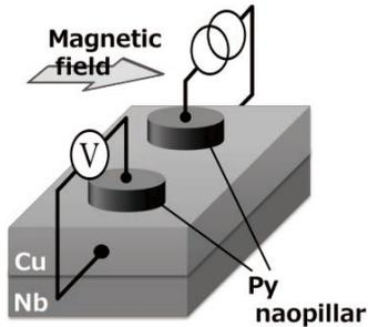
Figure 1: Sample structure and the probe configuration for measuring the spin signals.
