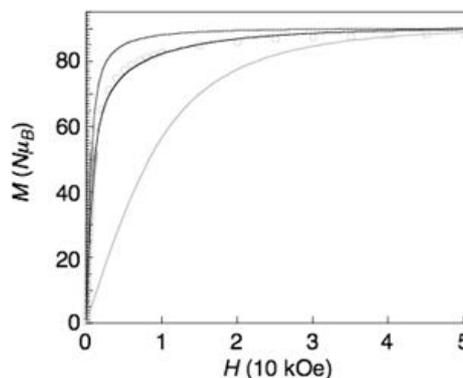
Figure 2: Magnetization vs. external magnetic field curve for **1**·18H<sub>2</sub>O at 2 K.
