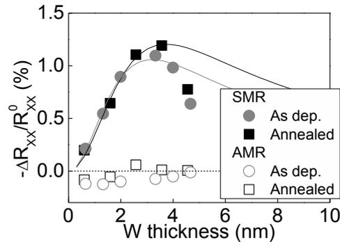
Figure 1: W layer thickness dependence on SMR (solid symbol) and anisotropic magnetoresistance (opened symbol) from annealed (square) and as deposited (circle) W/CoFeB/MgO heterostructures.
