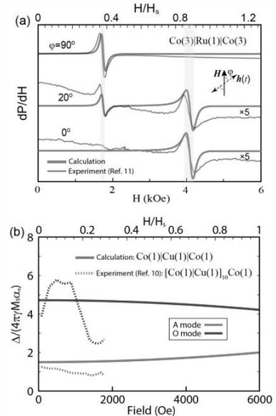
Fig.1: (a) Derivative of the microwave absorption spectrum [5] (b) Computed linewidths of the acoustic (A) and optical (O) modes [2].
