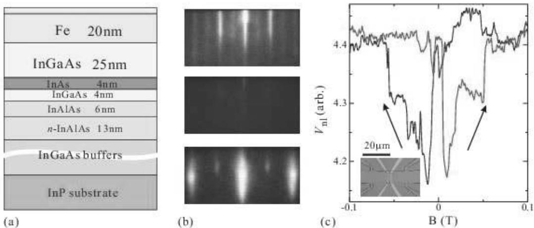
Figure 1: (a) Layered structure of MBE grown sample. (b) RHEED patterns. Top: (In,Ga)As surface. Middle: First monolayer of Fe. Bottom: 8nm thick Fe layer. (c) Non-local spin-valve voltage for spin-injection from Fe into InAs well. The inset shows a micrograph of the specimen.
