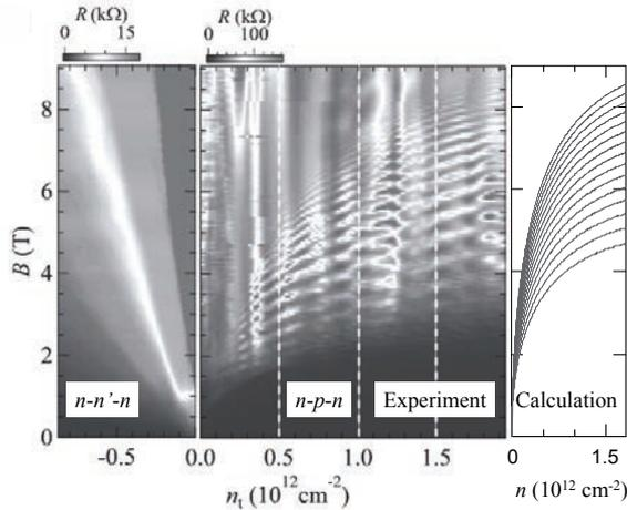
Fig. 1 Color-plot of two-terminal magnetoresistance of graphene n-n-n (left) and n-p-n (center) junctions. Simulated peak positions of carrier transmission between the counter-circulating quantum Hall edge channels at the pn interface (right).
