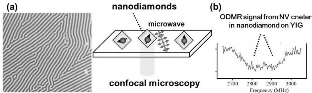
Figure 1: (a) polarization-microscope image of magnetic domains in the YIG film. (b) ODMR signal from NV center in nanodiamond on YIG.
