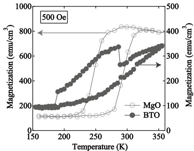
Fig. 1 Temperature dependence of magnetization of Ga-FeRh/MgO and Ga-FeRh/BTO structures.
