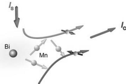
Figure 2: Illustration of inverse SHE in CuMnBi spin glass system. The pure spin current  $I_s$  is converted into the charge current  $I_c$  at the Bi site.  $I_s$  is also affected by fluctuating spins at the Mn sites. Red and blue arrows with green spheres are spins of conduction electrons ( $|e|$ ) and the curved arrows indicate the motions of spin-up and spin-down electrons.
