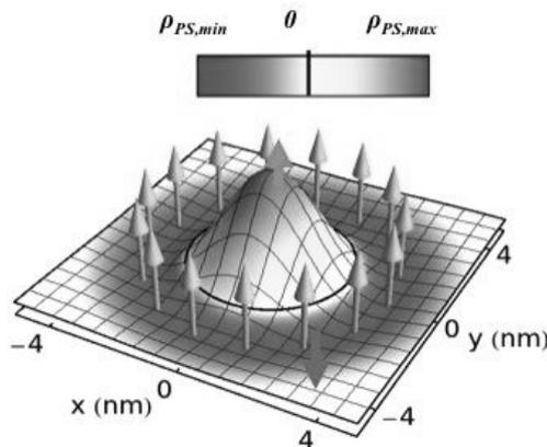
**Fig. 1** Spin corral. Colored surface: The hole-spin density  $\rho_{PS}$  of the pseudosinglet. Black circle indicates vanishing  $\rho_{PS}$ . Green arrows: Mn spins, placed to maximize the stability of the ferromagnetic alignment. Red and blue arrows: The more probable hole-spin projections at two positions [4].
