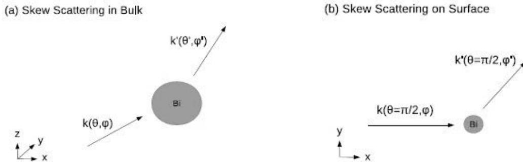
Figure 1: Schematic picture of skew scattering of conduction electrons by the Bi impurity in Cu bulk (a) and on a Cu surface (b). The Bi impurity has very extended state (large circle) in the bulk and a much more localized state (small circle) on the surface. The conduction electron in Cu is described by a three-dimensional wave vector in the bulk, and a two-dimensional wave vector on the surface
