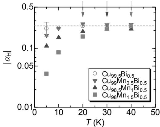
Figure 1: Spin Hall angles  $|\alpha_H|$  of CuMnBi ternary alloys as a function of temperature. The arrows indicate  $T^*$  where  $|\alpha_H|$  start to decrease. The broken line in the figure shows  $|\alpha_H|$  of  $\text{Cu}_{99.5}\text{Bi}_{0.5}$ .
