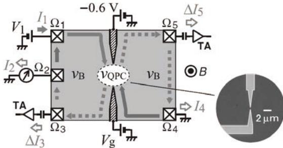
Figure 1: Schematic of a local FQH state ( $\nu_{\text{QPC}}$ ) sandwiched between bulk IQH systems ( $\nu_B$ ) and the measurement setup.
