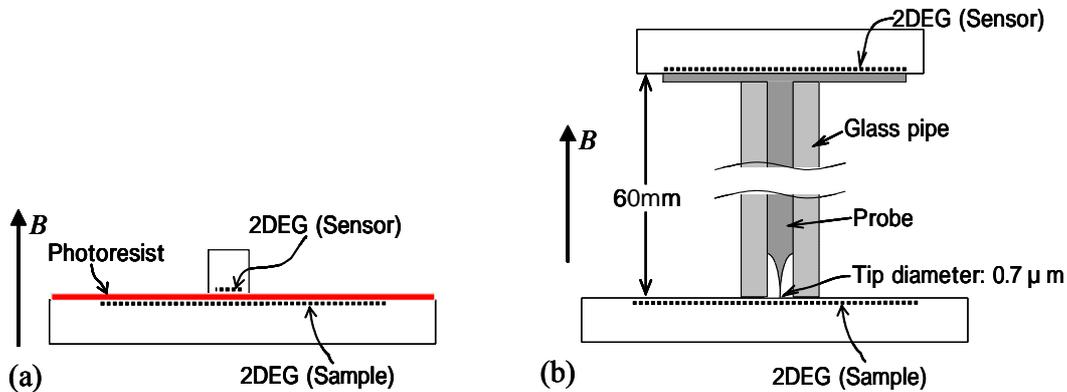
**Fig. 1** Schematics of the experimental setup for electrostatic potential imaging in (a) the previous scheme and (b) the presently developed scheme.
