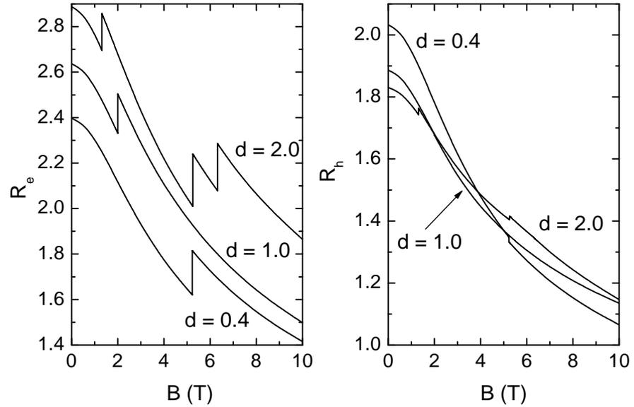
Fig. 2: The radii of the electron ( $R_e$ ) and hole ( $R_h$ ) lateral distributions in the quantum dots plotted versus the magnetic field strength  $B$  for a number of values of the inter-dot distances  $d$  measured in the effective Bohr radii  $a_B^* = 9.8$  nm. Abrupt jumps associated with the angular momentum transitions at certain magnetic field values (predicted in Fig. 1) are clearly visible. The response of the electrons is much stronger than that of the hole.
