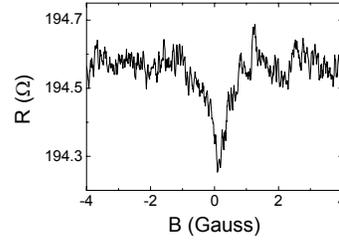
**Figure 2:** Low field magnetoresistance measured on a Hall bar made on the same heterostructure used to fabricate the rings. The minimum at zero field is due to weak anti-localization caused by Rashba SO interaction.
