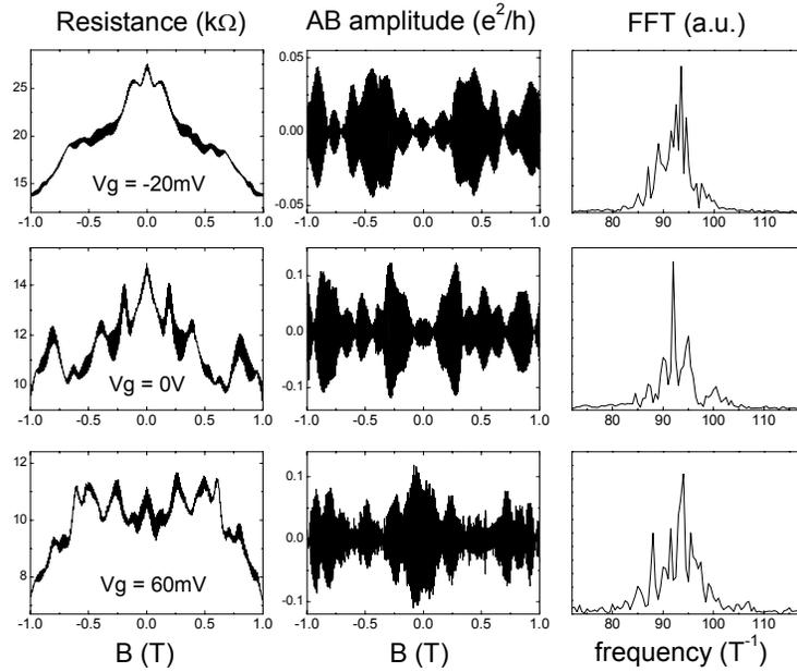
**Figure 3:** Gate-voltage dependence of the magnetoresistance (column 1), and its Fourier spectrum (column 3). The envelope functions of the AB oscillations are obtained by low frequency filtering of the  $R(B)$  curves, and are shown in column 2. We find that these three quantities depend strongly on the gate voltage, in a random way.
