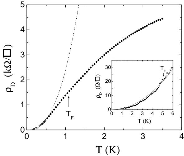
Fig 1:  $\rho_D$  vs  $T$  for  $p = 1.5 \times 10^{10} \text{ cm}^{-2}$ . Dotted line is the best  $T^{2.5}$  fit of the low temperature data. Data with open circles measured in dilution refrigerator. Inset:  $\rho_D$  vs  $T$  for  $p = 7.0 \times 10^{10} \text{ cm}^{-2}$ . Solid line is the best  $T^2$  fit.
