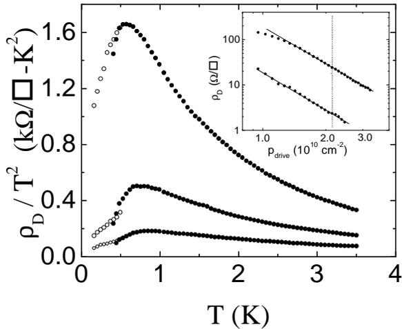
Fig 2:  $\rho_D / T^2$  vs  $T$  for from top to bottom  $1.5, 2.0,$  and  $2.5 \times 10^{10} \text{ cm}^{-2}$ . Inset:  $\rho_D$  vs drive layer density on log-log scale for the drag layer fixed at  $2.15 \times 10^{10} \text{ cm}^{-2}$  at  $T = 300$  (top) and  $80 \text{ mK}$ . Both data are well described by straight lines with slope close to  $-2.5$ . Matched density indicated by the dashed line.
