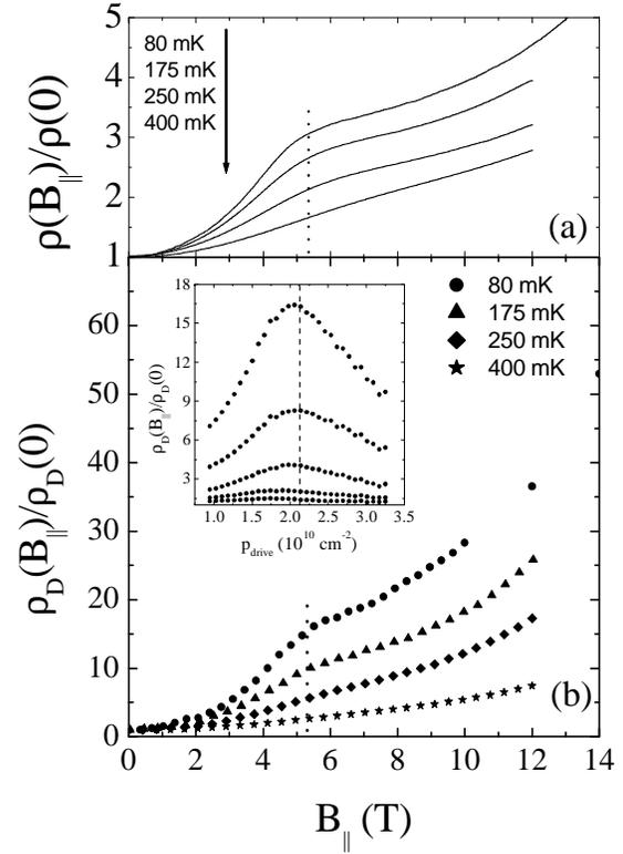
Fig 3: Normalized in-plane single layer magnetoresistance (a) and magnetodrag (b) at different temperatures for  $p = 2.15 \times 10^{10} \text{ cm}^{-2}$ . Inset (b): Normalized magnetodrag vs drive layer density for the drag layer fixed at  $p = 2.15 \times 10^{10} \text{ cm}^{-2}$ , for from top to bottom  $B_{||} = 14, 10, 5.3, 3,$  and  $2 \text{ T}$ .
