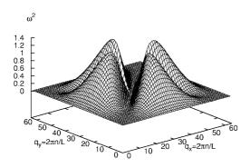
Fig. 2: Whole picture of phonon dispersion relations at critical temperature  $T_c \sim 0.33t_0/k_B$ . Only transeverse modes are plotted, and the condition for calculations are the same as above.
