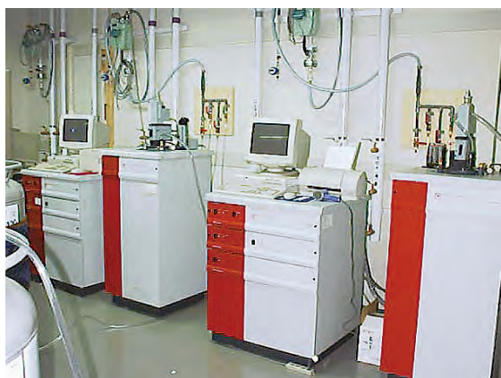
磁気特性測定装置 SQUID magnetometer (MPMS)
