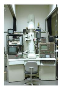
200 kV 電界放射形分析電子顕微鏡 200 kV electron microscope with an X-ray micro-analyzer
