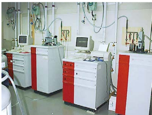
磁気特性測定装置 SQUID magnetometer (MPMS)
