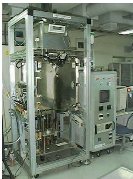
単結晶引上炉 Czochralski pulling apparatus with an induction heating system
