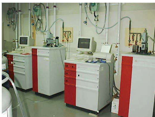
磁気特性測定装置 SQUID magnetometer (MPMS)
