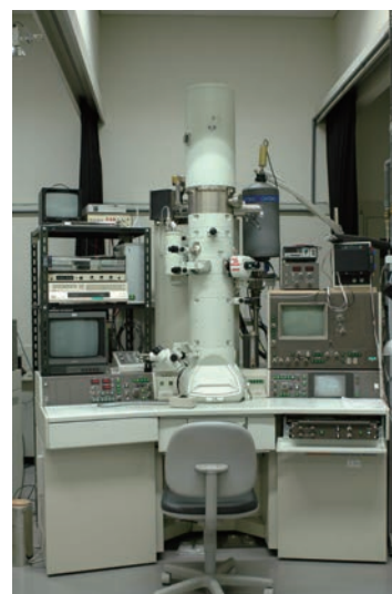
200 kV 電界放射形分析電子顕微鏡 200 kV electron microscope with an X-ray micro-analyzer
