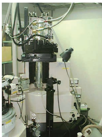
極低温用イメージングプレート型X線回折計 Imaging plate type X-ray diffractometer for low temperature application
