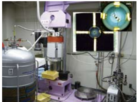
超高压物性測定装置「圧太郎」と試料部の拡大図。 Physical property measurement system under ultra-high pressure, "Oshitaro", and the enlarged sample part.
