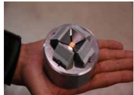
Fig.1 The palm cubic anvil cell.
