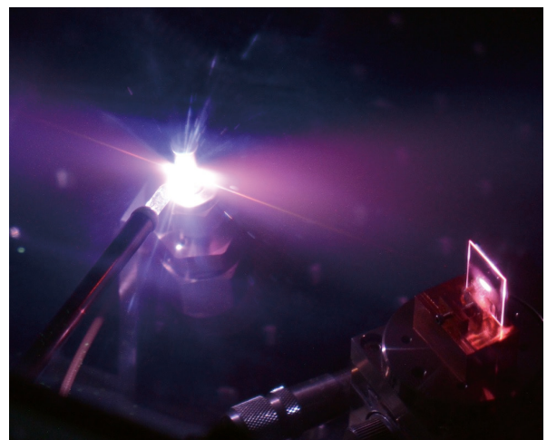
Fig. 5. 10-MHz high harmonic generation in an enhancement cavity.
