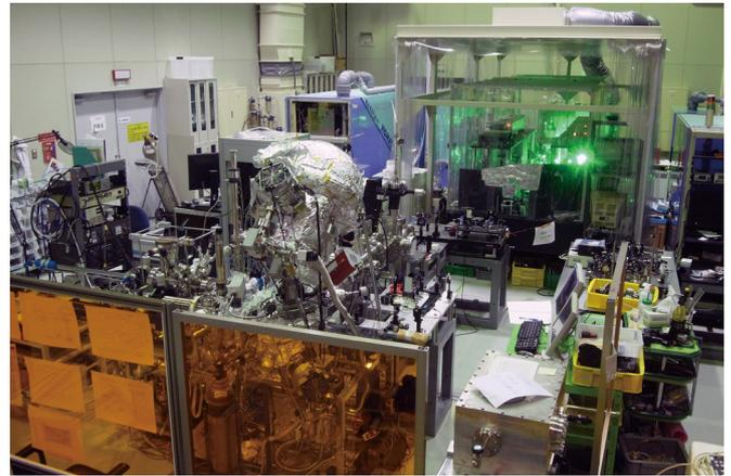
Fig. 7. Pump-probed photoemission system using 60-eV laser
