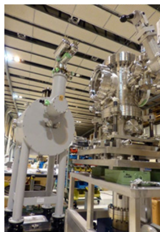
Fig. 4. Soft X-ray MOKE station
