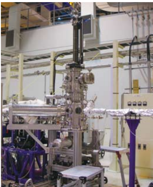
Fig. 1. Time-resolved soft X-ray spectrometer installed at BL07LSU
