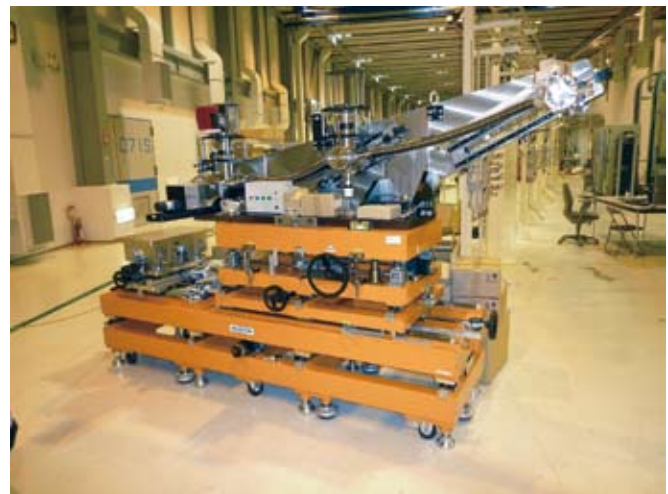
Fig.3. High resolution soft X-ray emission spectrometer at BL07LSU
