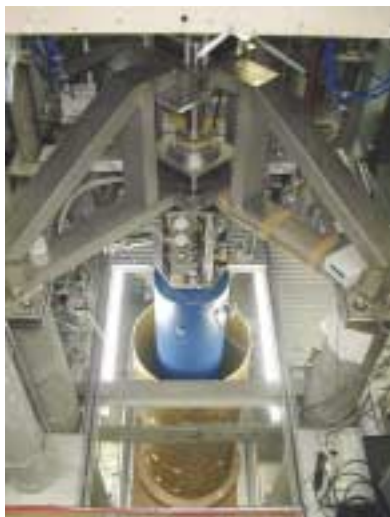
Fig. 1. ISSP ULT Rotation Cryostat with rotating scheme Tok-01. Two high precision air bearing units are located at the ends of the shaft. Electronics are located on a table above and driven by precision motor through timing belt. The connection between this table and the shaft which connects rigidly the cryostat is made by a soft torsion rod, which functions also as a rotational vibration isolator. Earth field cancellation coils are seen on a thick paper cylinder around the Dewar.
