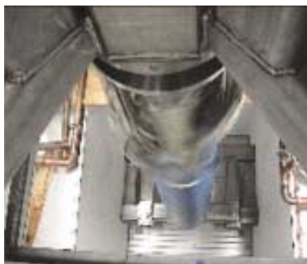
Fig. 2. ISSP High Speed Rotating Cryostat. Experiments under up to 6 rotation/sec are tested at dilution refrigerator temperatures.
