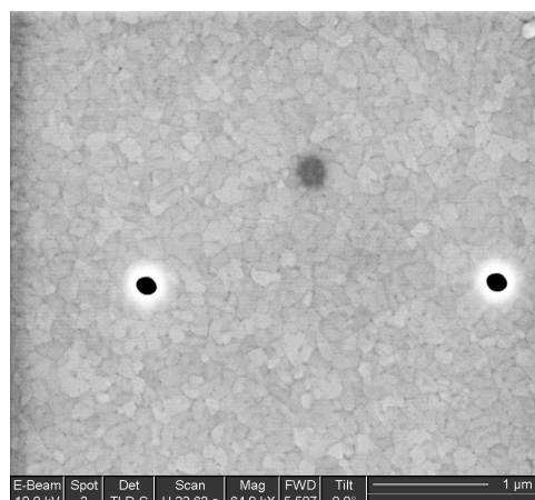
Figure 2. Double pinhole mask with center-to-center distance of 3 \mu\text{m} and the diameter of 170 nm.
