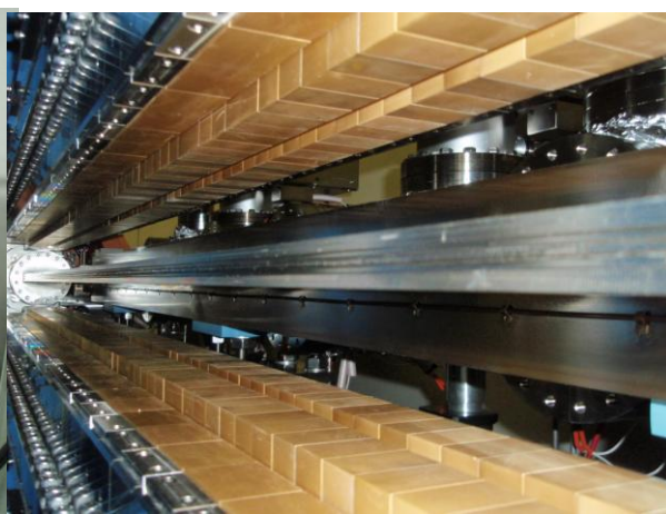
Fig.2 Arrangement of magnets in the figure-8 undulator of the vertically linear-polarization type.
