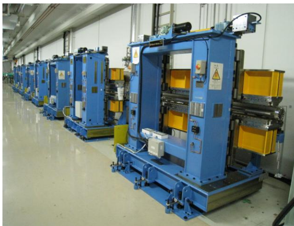
Fig.1 Eight figure-8 undulators in the SPring-8 storage ring
