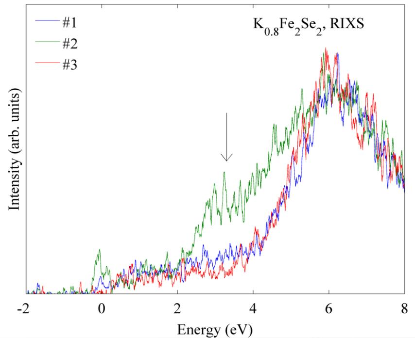
Figure 4: Time dependence of the Fe RIXS spectrum measured on  $K_{0.8}Fe_2Se_2$  for  $E_i = 712.5$  eV. The sample position was continually scanned for scans #1 and #3, and fixed for the first 10 minutes of scan #2 (one scan measurement time = 30 minutes).
