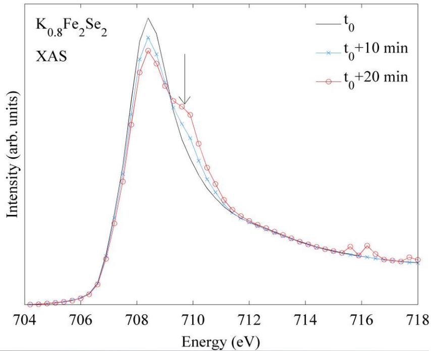
Figure 3: Time dependence of the Fe-L XAS spectrum measured on  $K_{0.8}Fe_2Se_2$  in the fluorescence yield mode. The sample position is fixed.
