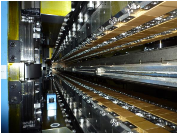
Fig.2 Arrangement of magnets in the figure-8 undulator.
