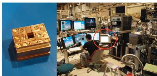
Figure 1. New sample holder for operando analysis (left) and actual condition of the 3D nano-ESCA measurements (right). The semiconductor parameter analyzer is shown in a red circle.
