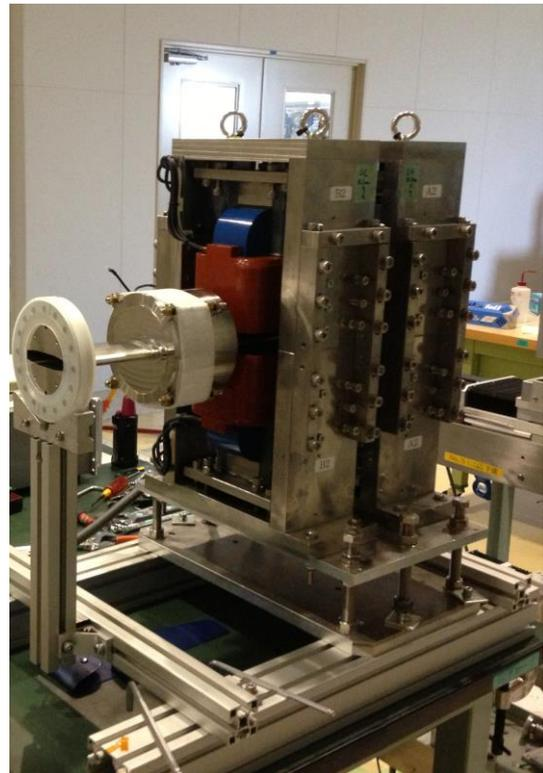
**Figure 1.** Adjustment of the electromagnetic phase shifter before the reinstallation in the SPring-8 storage ring.
