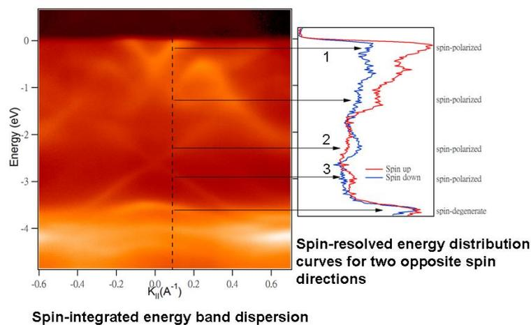
Fig.3: The correspondence between angle-resolved photoemission spectra and spin-resolved photoemission spectra for 5 ML PbAu alloy/Ge(111) at RT
