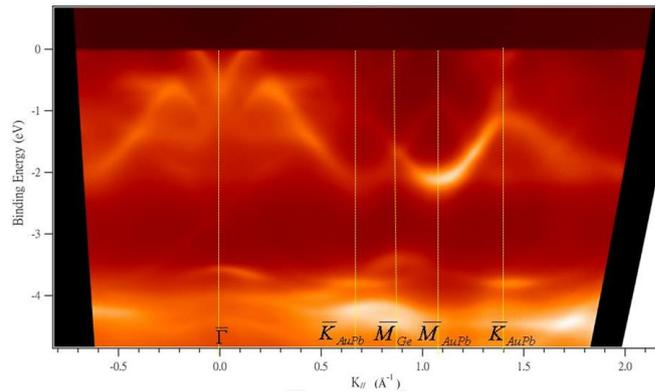
Fig.2: The angle-resolved photoemission spectra of energy band dispersions for 5 ML PbAu alloy/Ge(111) at RT
