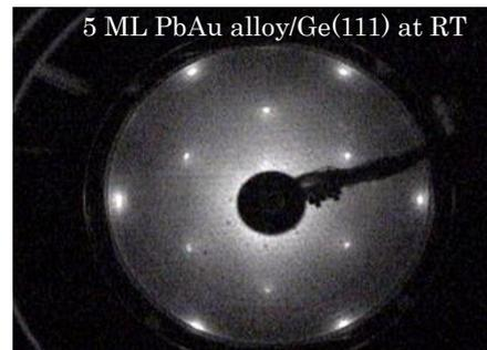
Fig. 1: The LEED patterns of 5 ML Pb /Au/Ge(111)- $\sqrt{3}\times\sqrt{3}$  R30° at LT and 5ML PbAu alloy/Ge(111) at RT
