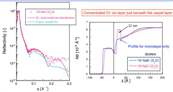
Fig. NR profiles with fitting curve in which Cl<sup>-</sup> ion distribution is considered. (left) Scattering length density obtained by the fitting. (right)
