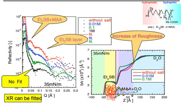
Fig. NR profiles and scattering density profiles for poly(Et<sub>2</sub>SB-*d*<sub>10</sub>)<sub>23</sub>-*b*-poly(MAA)<sub>49</sub> monolayer on subphase with different NaCl concentrations of 35mN/m.
