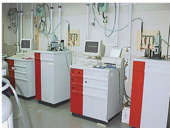
磁気特性測定装置 SQUID magnetometer (MPMS)
