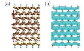
Figure 1: (a) Current density in 8-zigzag graphene nanoribbon with an antiferromagnetic junction under a finite bias voltage of 0.3 V. (b) Isosurfaces of the a-component of that.
