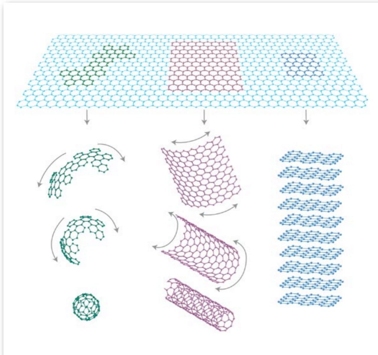
From the 2D graphene, “scissoring and wrapping” can give rise to 0D bucky balls, 1D nanotubes and 3D graphites.
