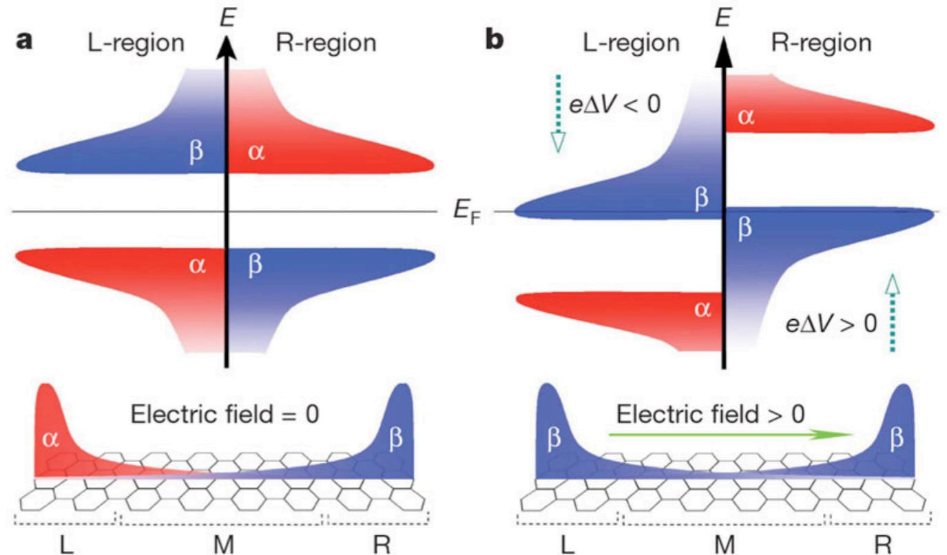
Using **electric field** to manipulate the magnetic properties in **zigzag graphene nanoribbon**.
