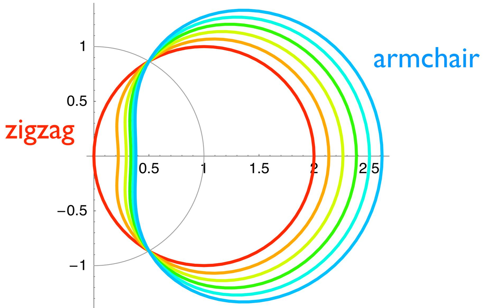
Contours in the complex  $z$ -plane for nanotubes with different chiralities (from zigzag to armchair).
