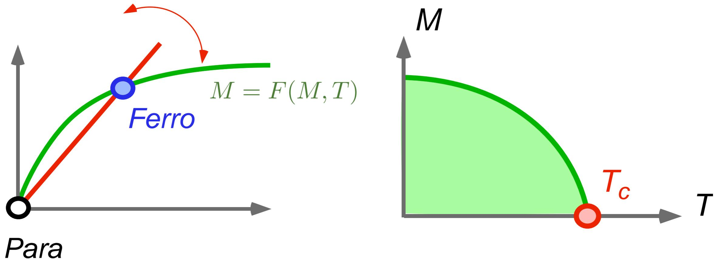
In Weiss mean-field theory, the magnetization is determined by some **self-consistent equation** and often changes **continuously** with temperature and other parameters.
