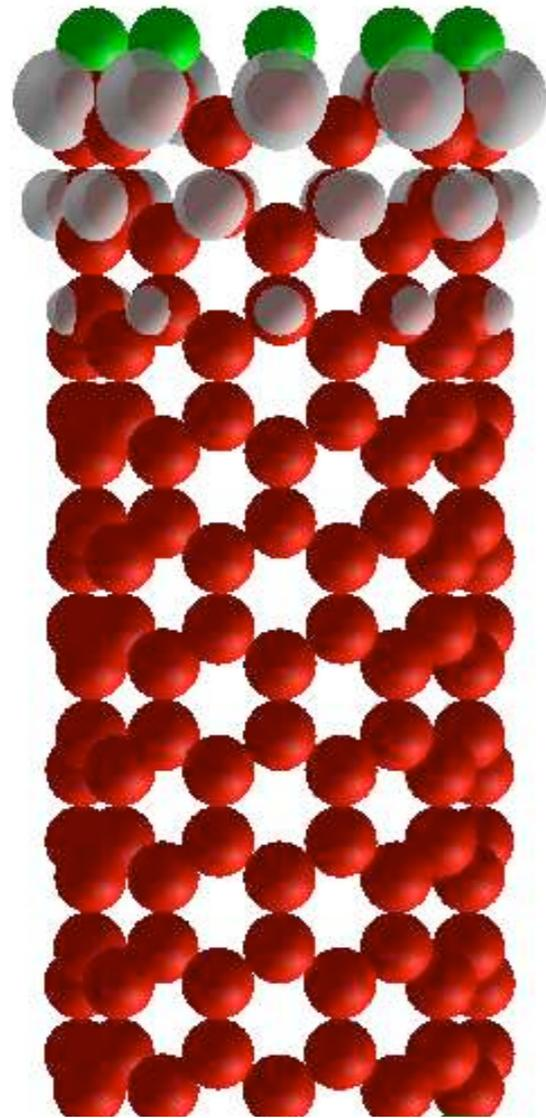
We found the ground state of the semi-infinite carbon nanotube has **quantized magnetic moment**,
