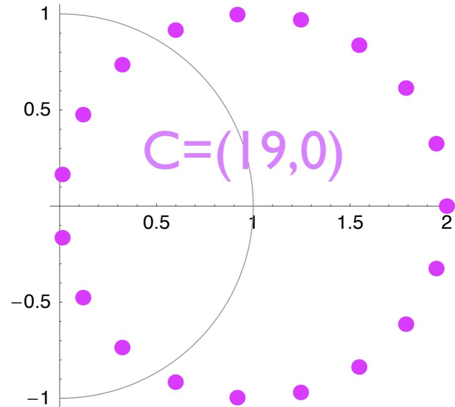
In fact, for nanotubes with **parallel chiral vectors**, the solutions fall onto the **universal contour** in the complex plane.
