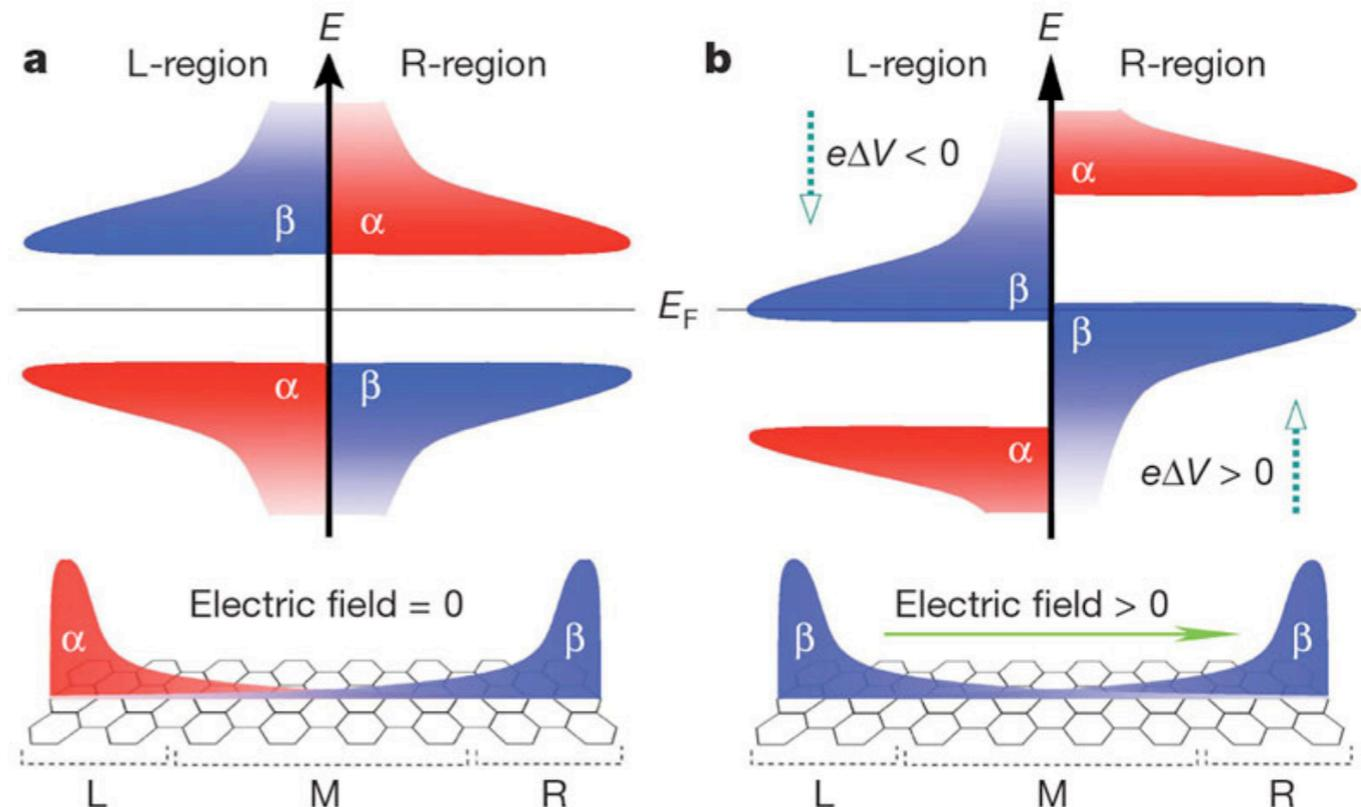
Using **electric field** to manipulate the magnetic properties in **zigzag graphene nanoribbon**.
