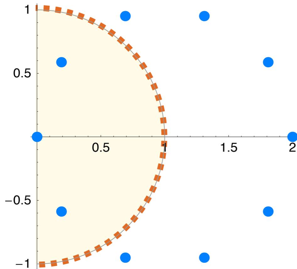
Taking  $(10,0)$  zigzag carbon nanotube as an example, there are **ten solutions** in the complex plane. Only **three** of them are decaying modes with  $|z| < 1$ .
