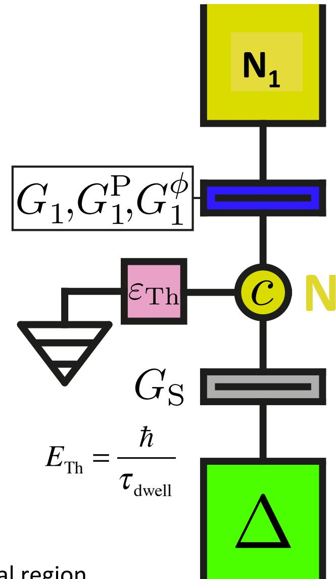
Measure of coupling strength: **Thouless energy**  $E_{\text{th}}$
