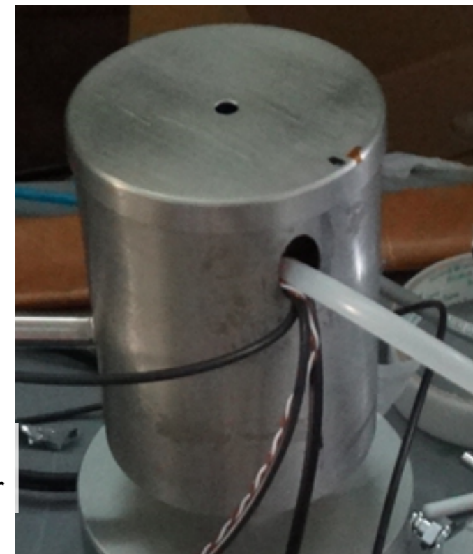
Magnetic shield inside: 20\text{nT}
