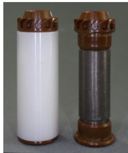
Capsule ( \phi 8\text{mm} ), Sample ( \phi 6 \times 20 \text{mm} )
