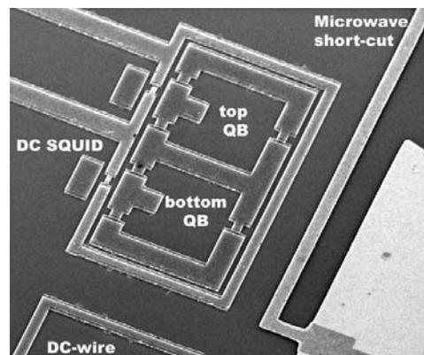
Fig. 3. Two coupled flux qubits. The qubits are surrounded by the SQUID loop.
