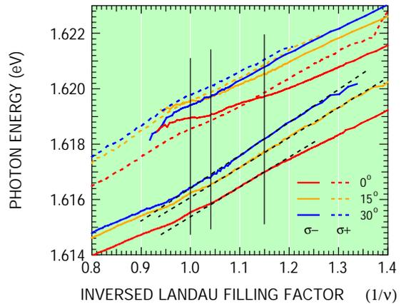
Fig. 3. Inversed Landau filling factor dependence of emission peak energies in tilted field configuration for both circular polarizations.
