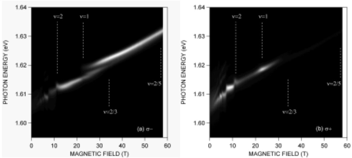
Fig. 1. Streak image view of photoluminescence spectra vs. magnetic field in the modulation-doped n-type CdTe/(Cd, Mg, Mn)Te quantum well at 1.5 K for a)  $\sigma^-$  polarization and b)  $\sigma^+$  polarization.
