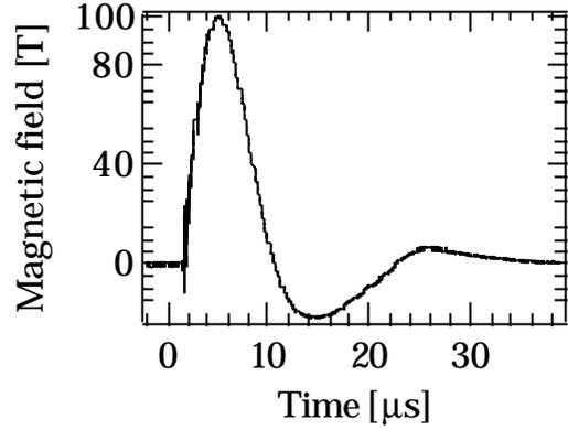
**Fig. 2.** Waveform of the magnetic field generated by single-turn coil technique. The magnetic field is generated within 10  $\mu\text{s}$ .
