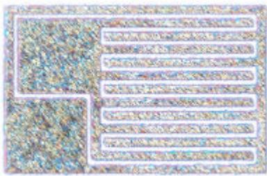
**Fig. 4.** ( $\omega$ ) Top view of the sample. 2DES exists between inner contact and outer contact.
