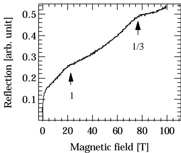
**Fig. 5.** ( $\zeta$ ) Real part of reflectivity as a function of the magnetic field (for bias frequency of 350 MHz and initial temperature of 4.2 K). In the low magnetic field ( $B < 10$  T), structures of  $V_{ref}$  were observed corresponding to the integer quantum Hall effect. In higher magnetic fields, reflectivity shows monotone increase and two
