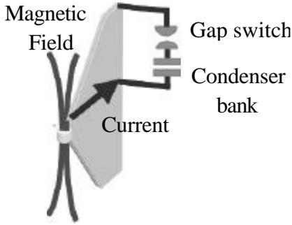
**Fig. 1.** Single-turn coil technique of ultra-high magnetic field generation. Ultra-high magnetic fields are generated by directly discharging current from a fast condenser bank to a single-turn coil.
