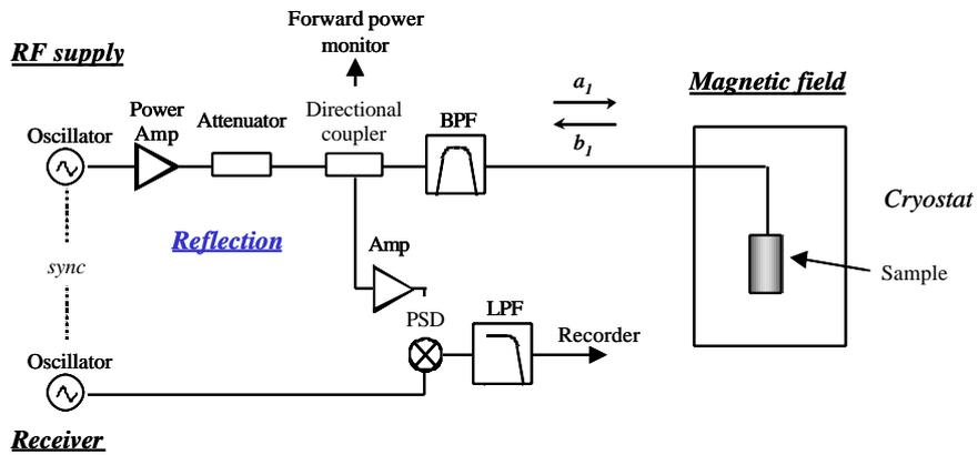
**Fig. 3.** Schematic diagram of RF reflection measurement system. Noise and induced voltage component in reflected signals were first eliminated by the band-pass filter. The signal is amplified using the signal amplifier and detected by a phase sensitive detector (PSD). The PSD output signal is recorded on recorders.
