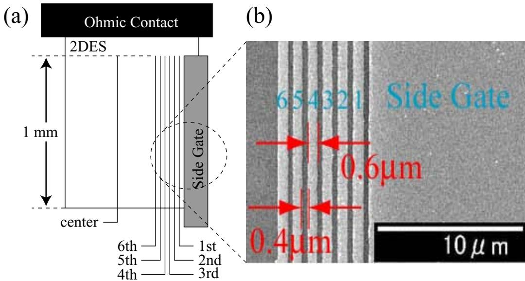
Figure 1: (a) Schematic view of the sample. (b) The SEM image of the side gate and wire gates. The thin wire gates (1 ~ 6) are used with the local capacitance measurements. By applying negative bias voltage to a side gate, the confinement potential is formed near the side gate boundary.
