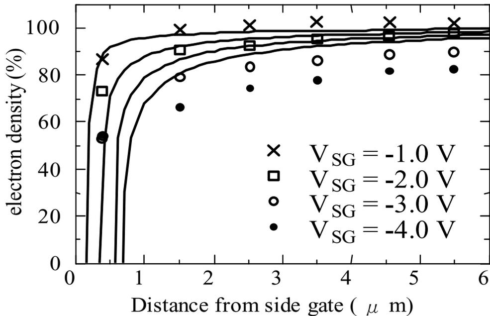
Figure 2: Electron distribution at the several  $V_{SG}$  near the sample boundary normalized by a bulk electron density. The dots in the figure are experimental results evaluated by the magnetocapacitance measurements. The curves are calculated ones by using the theoretical model [1].
