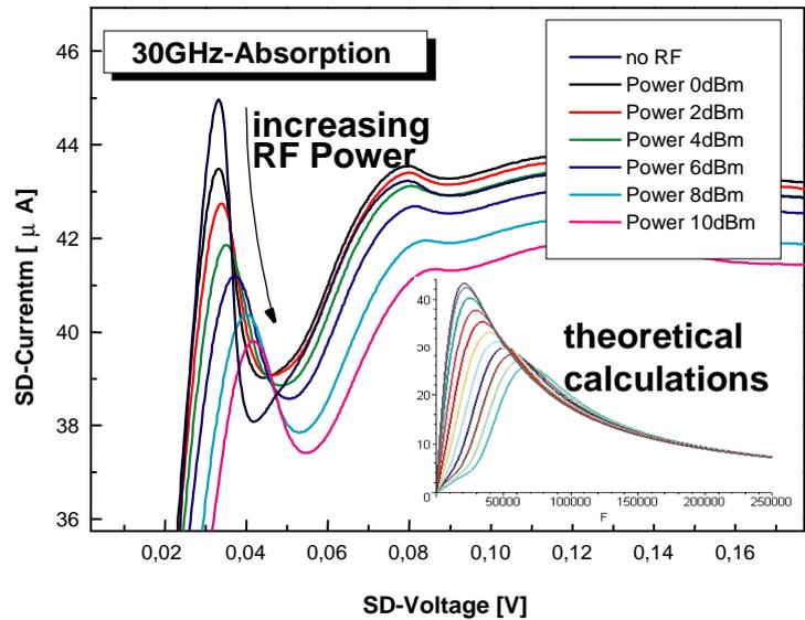
figure 4: I-V-characteristics with RF-Field
