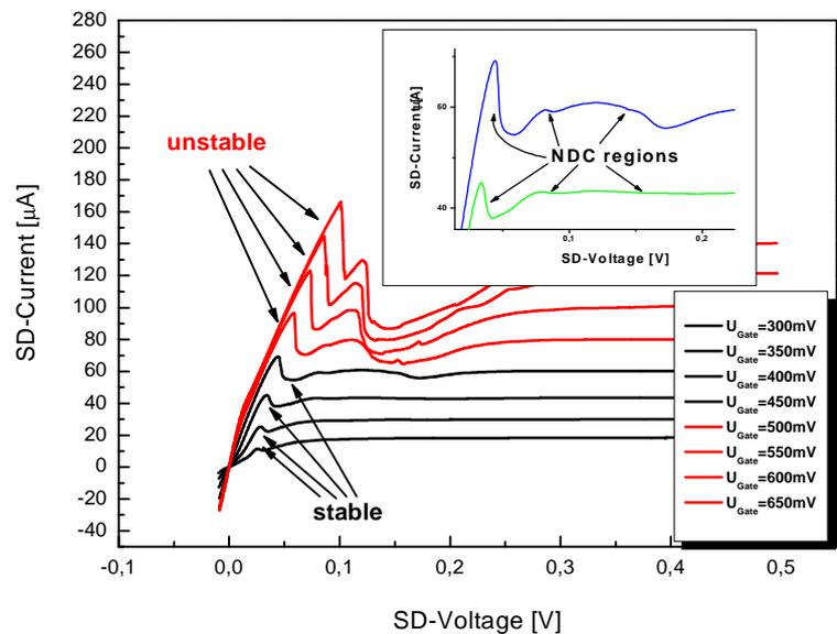
figure 2: I-V-characteristics
