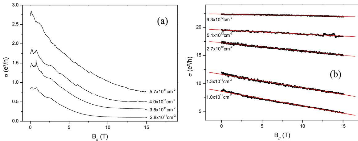
**Figure 1 :** In-plane magnetoconductance for various electronic densities, at  $T=50mK$  : a) For the low densities, b) for the higher densities.
