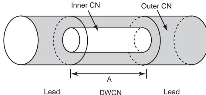
Figure 1: Schematic illustration of two-terminal DWCN. The inner tube is finite with the length  $A$  and the outer tube is infinitely long and connected to reservoirs. In the region without the inner tube, the outer tube plays a role of ideal leads.
