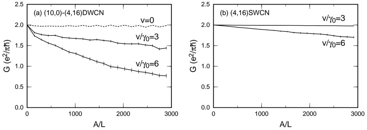
Figure 2: Conductance for (a)(0,10)-(4,16) DWCN and (b)(4,16) SWCN's as a function of the length  $A$  at the energy  $EL/2\pi\gamma=0.2$  where  $2\pi\gamma/L$  is the bottom of the first excited subbands measured from the Fermi energy  $E=0$ . In this case,  $L=4\sqrt{2}a=45.1\text{\AA}$ . A dotted line in (a) is the conductance in the absence of impurities.
