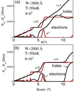
Magnetoresistance of a 2000 Å PQW with **2D** hole gas as a function of the normal component of the magnetic field for different tilt angles  $\Theta$  between the applied magnetic field and the normal to the plane of the substrate at T = 50 mK. The in-plane magnetic-field component is directed along the y axis, perpendicular to the current flow.
