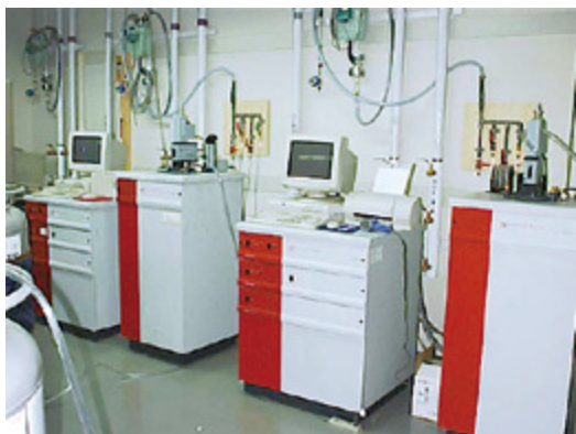
磁気特性測定装置 SQUID magnetometer (MPMS)
