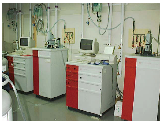
磁気特性測定装置 SQUID magnetometer (MPMS)
