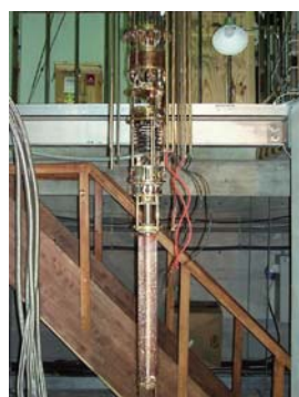
Fig.1 強磁場・核断熱消磁冷凍機 A large nuclear demagnetization refrigerator in high magnetic fields.
