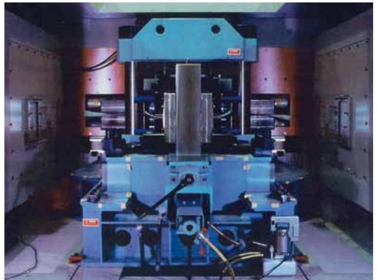
爆破保護室内に設置された「電磁濃縮法」による超強磁場発生装置。 An ultra high-magnetic-field generation system using the electromagnetic flux compression method has been installed at ISSP inside protection housing.
