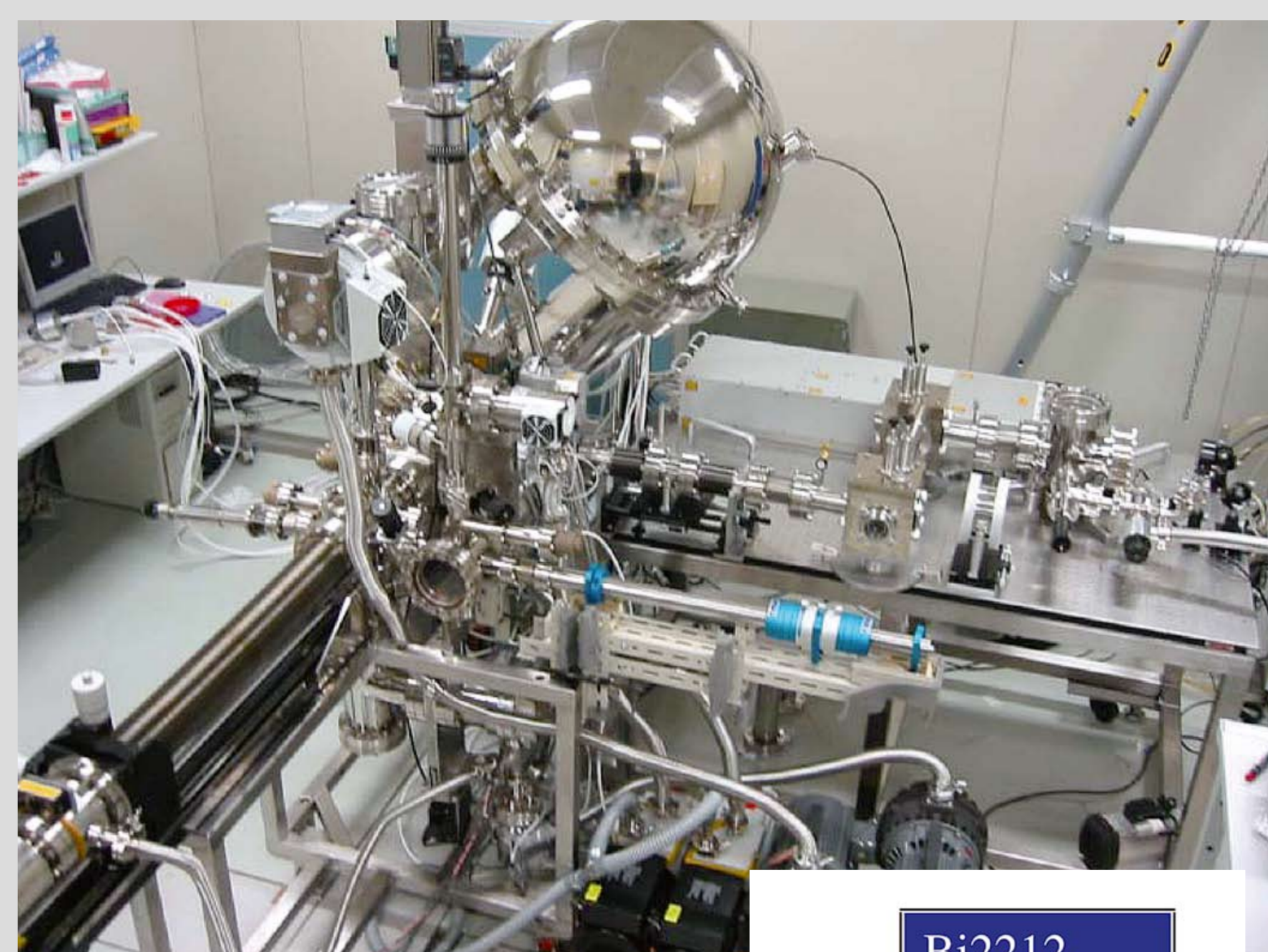
世界最高の分解能を持つレーザー光電子分光装置と高温超伝導体のバンド分散。 Laser-based photoemission spectrometer with the world's highest energy resolution. The inset shows the observed band dispersion of a high-Tc superconductor.
