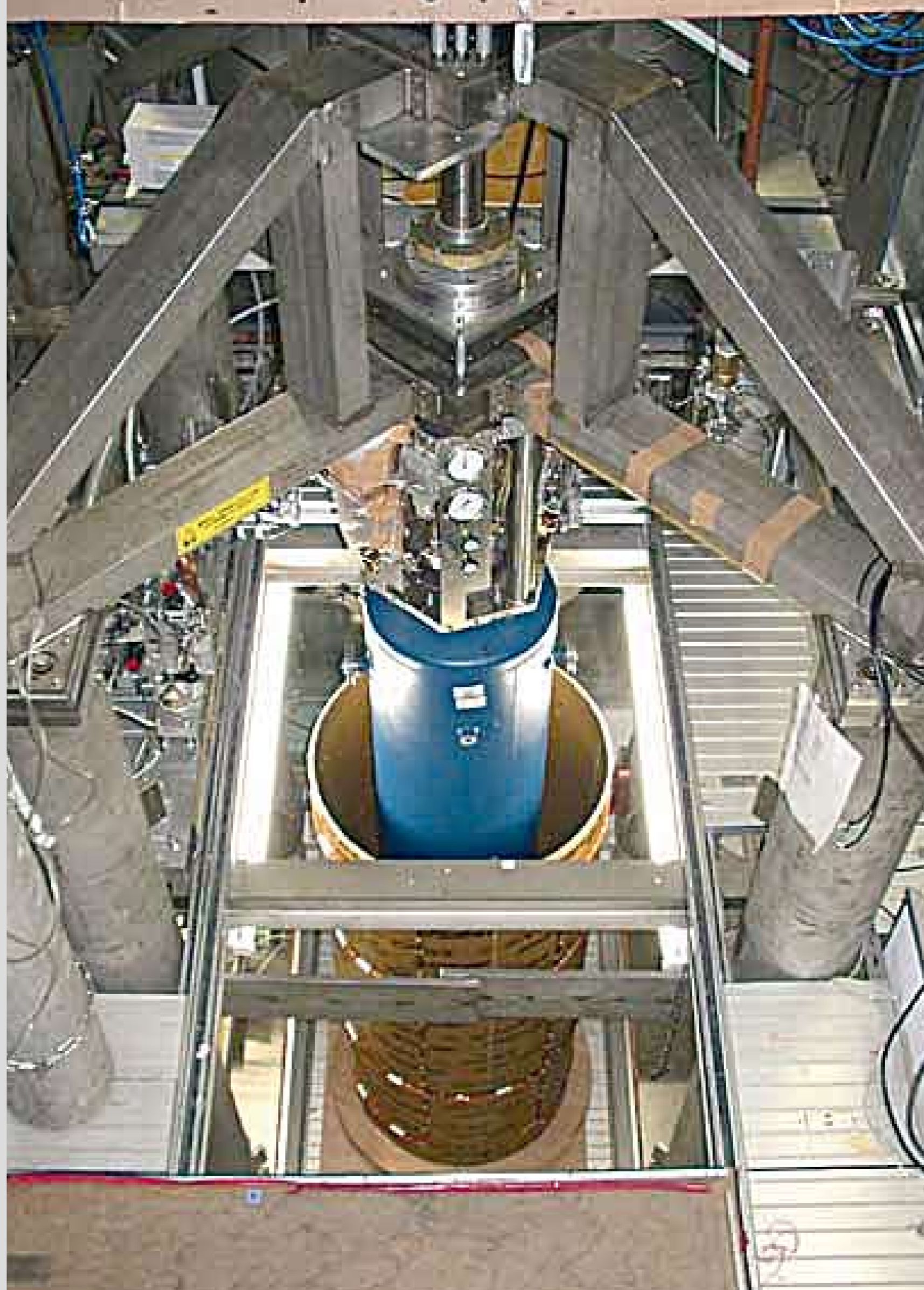
毎秒2回転までの定常回転状態の下で数百マイクロケルビン迄の超流動観測が行われている世界最高速の「ISSP超低温回転クライオスタット」。 ISSP ULT rotating cryostat with world's highest rotation speed. The physics of vortices and textural transitions in superfluid 3 He is being studied under steady rotation with the speed up to 12 rad/s.
