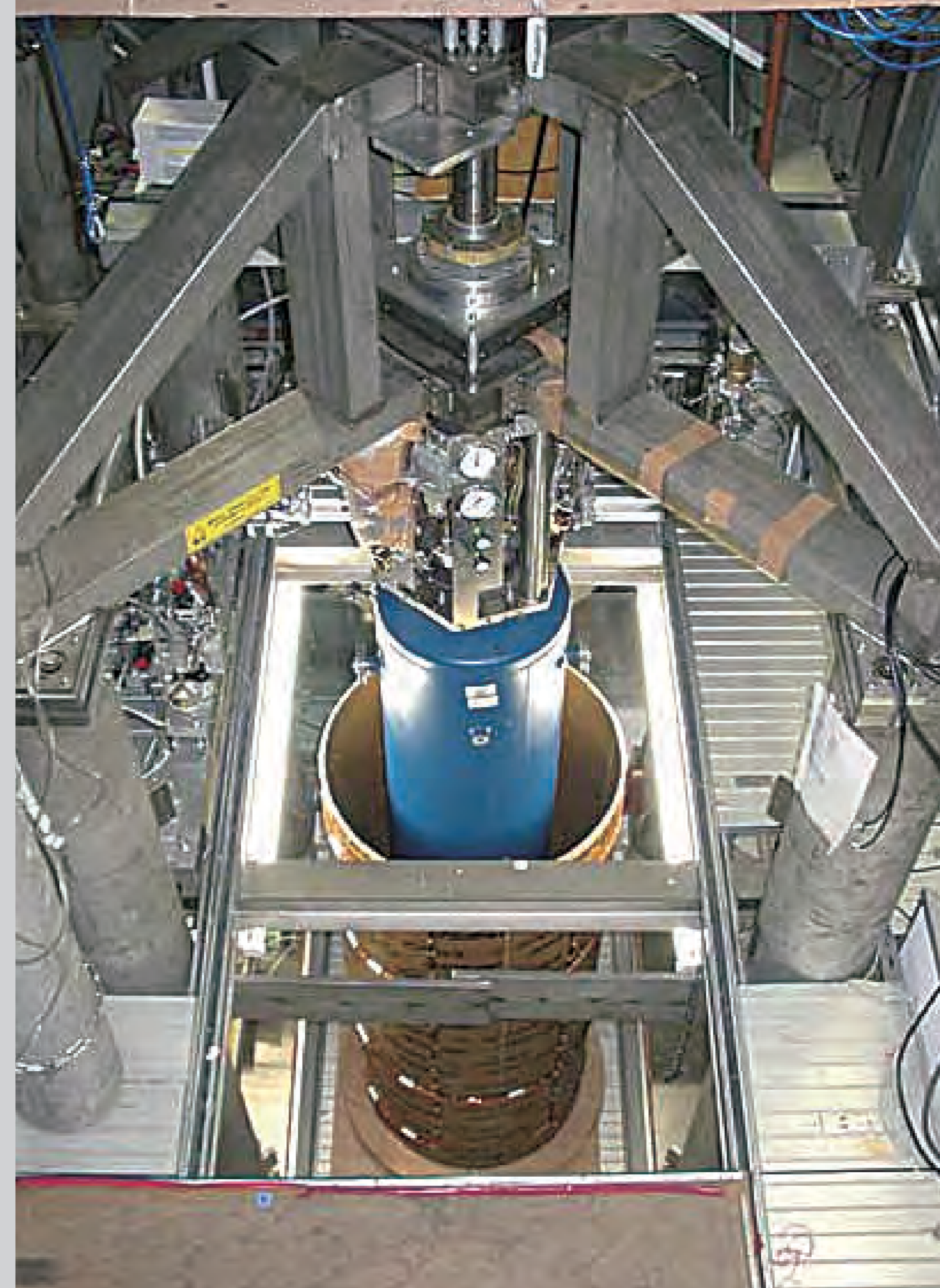
毎秒2回転までの定常回転状態の下で数百マイクロケルビン迄の超流動観測が行われている世界最高速の「ISSP超低温回転クライオスタット」。 ISSP ULT rotating cryostat with world's highest rotation speed. The physics of vortices and textural transitions in superfluid 3 He is being studied under steady rotation with the speed up to 12 rad/s.
