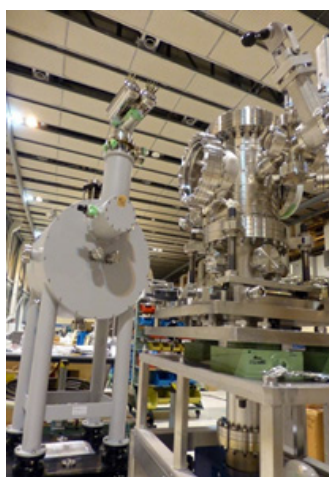
Fig. 4. Soft X-ray MOKE station
