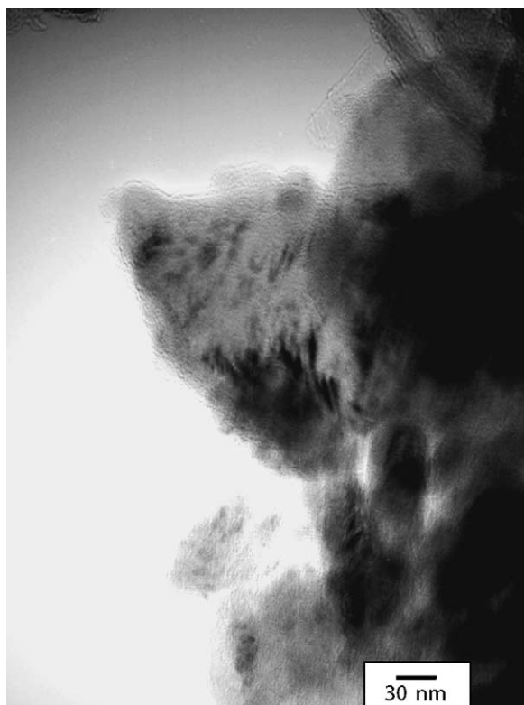
Fig. 4. TEM micrograph of TiH 2 /graphite mixture milled for 126 min.
