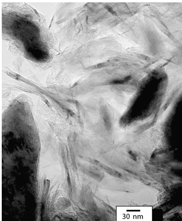
Fig. 3. TEM micrograph of TiH 2 /graphite mixture milled for 30 min.
