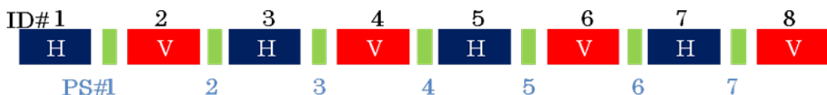
Figure 1 Schematic of a new undulator at SPring-8 BL07LSU
